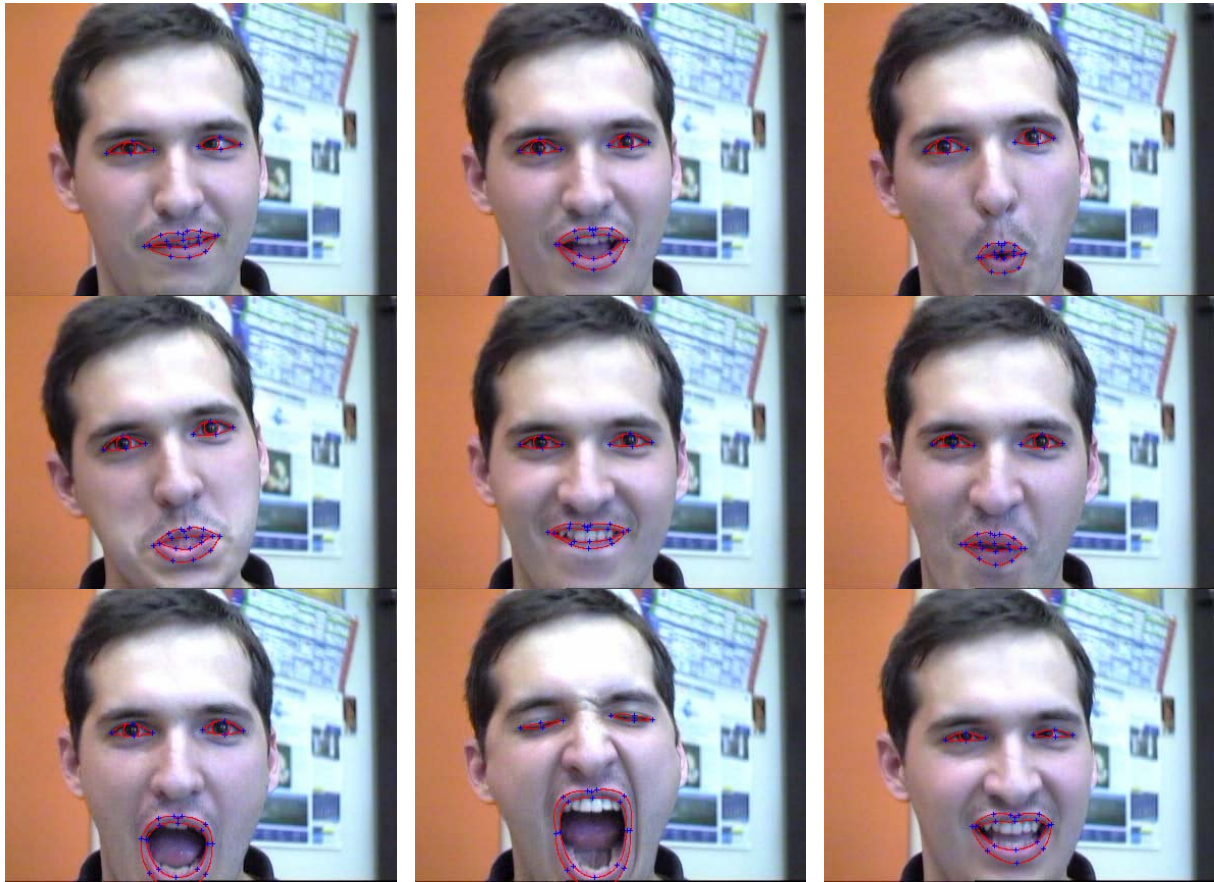
Figure 1 – Automatic eye and mouth motion capture in video sequences using deformable templates.
